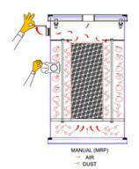
The Manual Reverse Purge (MRP) System allows the operator to not have to open the vacuum cleaner in order to clean the Cartridge. By opening the Reverse Purge Atmospheric Pressure Release Valve the Cartridge is automatically purged of dusts. This Purging System reduces maintenance down time.
